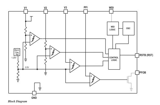
The SP6336/6337/6338 family includes a low-voltage precision bandgap reference, three precision comparators, an oscillator, a digital counter chain, a logic control block, trimmed resistor divider chains and additional supporting circuitry. The family is designed to supervise up to 3 independent supply voltages. V1 and V2 supply inputs have their resistor dividers on the chip. Their trip thresholds are factory trimmed. V3 input allows users to customize an
